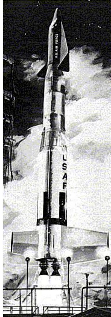
Early plans for the X-20 Dyna Soar called for sub-orbital tests using a modified Titan I ICBM. (USAF)
