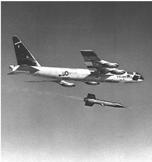
An XLR-11 equipped X-15 being dropped from a NB-52 at the beginning of a test flight. (NASA)
