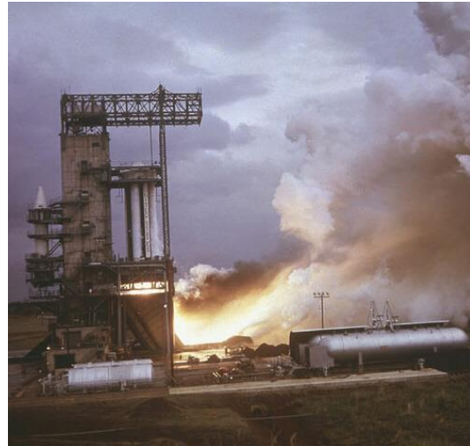
The SA-T undergoing a static test firing. (NASA)
