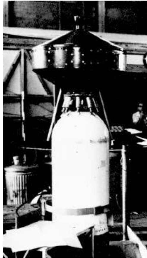
A USAF lunar orbiter attached to the final stage of its Thor-Able launch vehicle (NASA)
