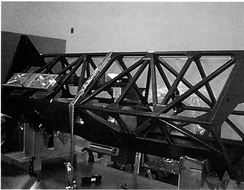
Figure 8: This is an optical bench mockup of the Advance Camera for Surveys that will be installed in the Hubble Space Telescope during the third service mission scheduled for 1999. It will have more advanced detectors than Wide Field Planetary Camera 2 and a coronagraphic capability. It should be capable of making efficient searches for and observations of faint companions in visible wavelengths.
