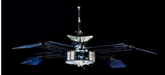
Mariner 4 made the first successful flyby of Mars in 1965 returning 21 images taken with the camera visible underneath. This same basic design served as the basis of most American planetary probes for more than a quarter century. (JPL/NASA)
